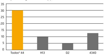
The table shows the toughness of Toolox $^{\circ}$  44 compared to some standard steels that are heat treated to 45–55 HRC. Toughness values for Toolox $^{\circ}$  at -20 $^{\circ}$ C are stated in the product certificates.
