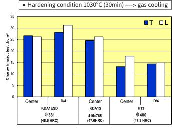
Charpy impact test compering result (normal temperature • 2mm U notch)
